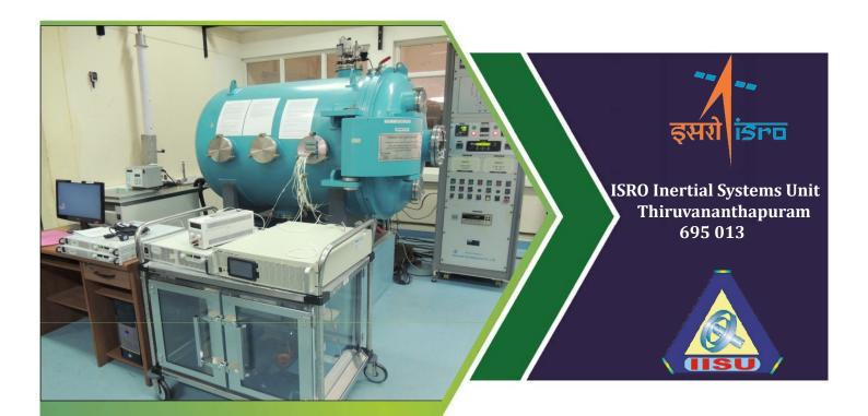
Thermovacuum testing on inertial systems used in launch vehicles and spacecrafts
