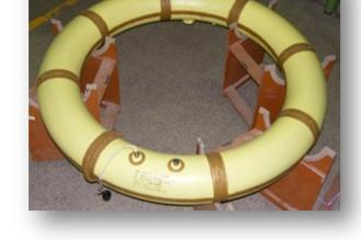
connecting rings. The shells are welded to the rings by TIG welding process.
